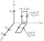
**EVALUATE** Consider a corresponding loop in the x-z plane, as shown above. Then  $-\partial E_z/\partial x = -\partial B_y/\partial t = 0$ , since there is no  $B_y$  by assumption. Thus  $-\partial E_z/\partial x = 0$ , and  $E_z$  must be a constant, so it cannot be part of the wave.
